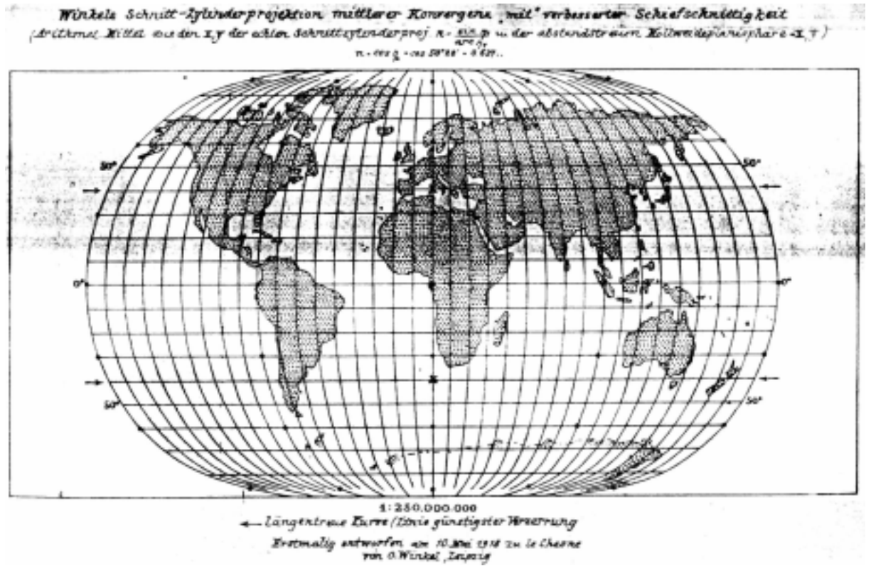
Fig. V: Winkel's secant cylindrical projection of mean convergence (arithmetic average of x, y of the true secant cylindrical projection and the equidistant Mollweide planisphere)
