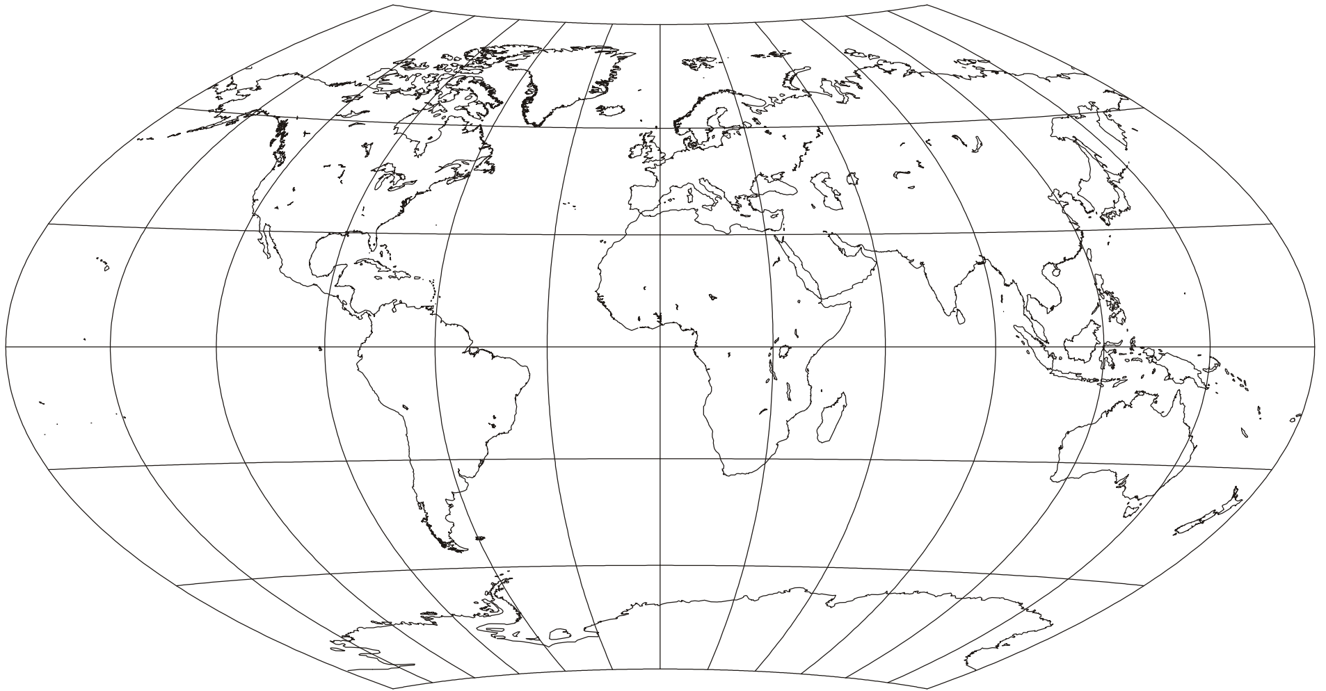
Wagner IX (or Aitoff-Wagner); Azimuthal (Arbitrary Modified Aitoff) Neither Conformal or Equal-area; K. H. Wagner; 1949
